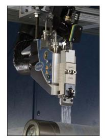
Saturn solenoids are designed specifically for Nordson pneumatic hot melt adhesive dispensing guns. These balanced, 3- and 4-way piloted valves deliver maximum shifting force in both directions by alternately supplying air to each end of the spool. Equal shifting forces at energization and de-energization result in resistance-free shifting, increased reliability and faster, more consistent response times.
