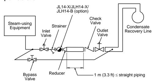
NOTE: Be sure to size outlet piping large enough to accommodate any flash steam that may form to prevent any increase in back pressure. (Outlet pipe size should always be properly calculated, contact TLV for assistance.)
