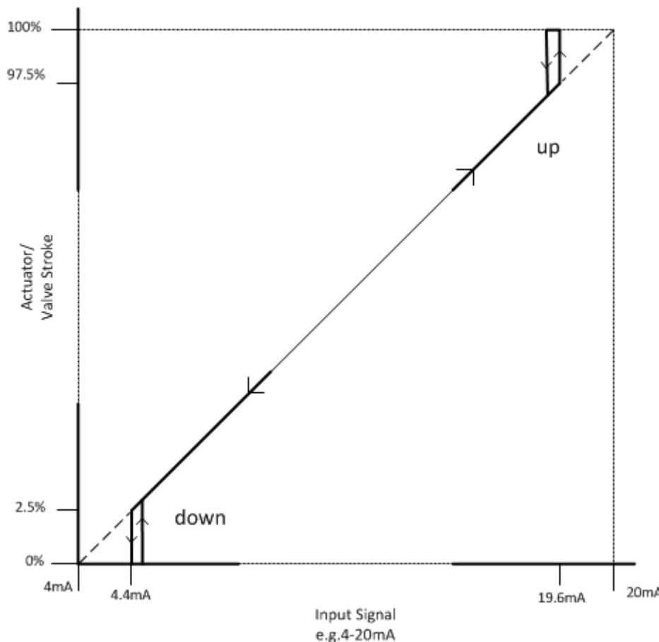
The Close Tight Function (default disabled) ensured that the actuator securely reached the limit positions up /down - (actuator switched off via limit or torque switch). Adjustable range: 0.5%...5.0%.
