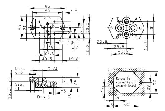
Subplates size 6 with interface to DIN 24 340-A 6 and ISO 4401-AB-03-4-A Cat. No. 1065183 G 3/8
