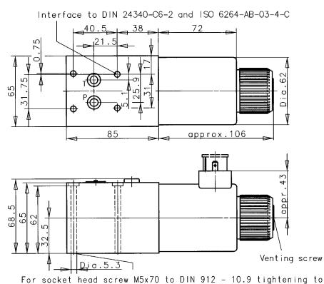
For socket head screw M5x70 to DIN 912 - 10.9 tightening torque 7.6 Nm The mounting screws are not included in the delivery.
